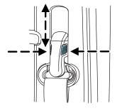
**WARNING:** Position the safety belt height adjusters so that the belt rests across the middle of your shoulder. Failure to adjust the safety belt properly could reduce the effectiveness of the safety belt and increase the risk of injury in a collision.
